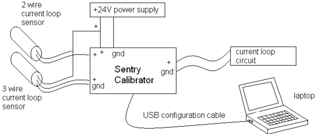
Either two wire or three wire current loop sensors can be used. The output is two wire current sourcing and can accommodate almost any application including most three wire circuits. The Sentry calibrator is placed in series between the sensor and the circuit the sensor would normally be connected to.
