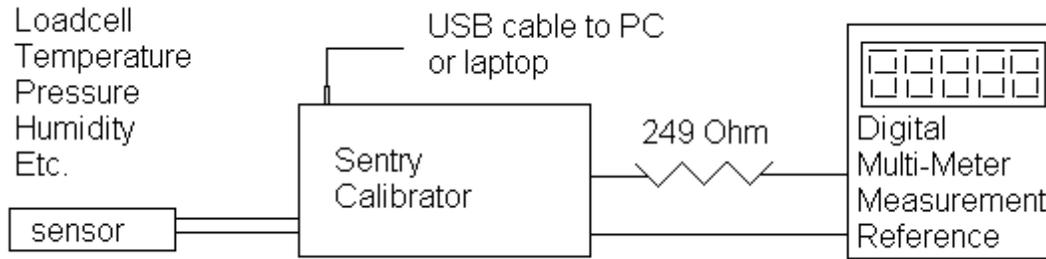
The following procedure can be used to program the Sentry Calibrator;
