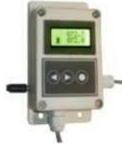
The Sentry Process Controller monitors a sensor output (voltage or current), displays a reading in user determined units, and operates a relay if the threshold set point is surpassed.
